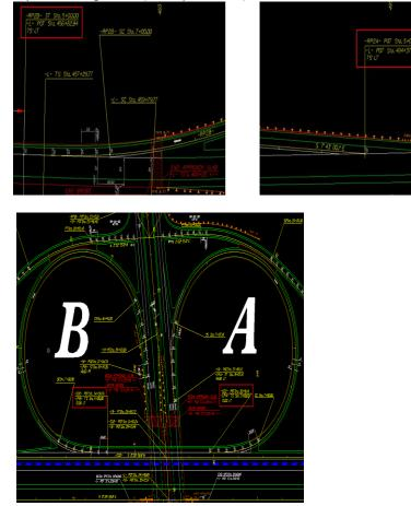
3. "Angular Exits" (2° 18' to 4° 07') and "Parallel Entrances" are common ramp design, but not always. The bearing at the POB and POE of loop alignments (also CD, directional median crossovers, and detours) should be paralell to their respective offsetting chain. See Roadway Standard Drawings 225.03 for other scenerios.
